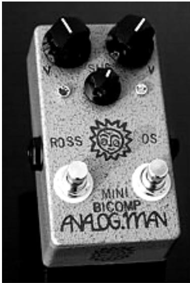
This product is actually two effects pedals in one. The left side is based on an improved version of the Ross compressor (compROSSor) and the right side the Dan Armstrong Orange Squeezer (Juicer). Each is independent and can be used separately or together. The order of the pedals, if used together, is Juicer first. Here are the basic specifications:
