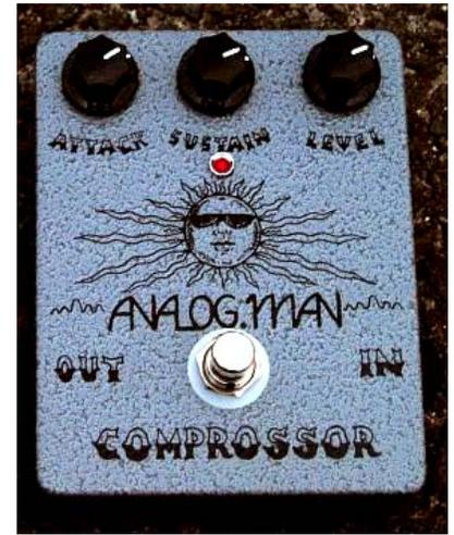
**JACKS:** Right is input, left output. Battery is disconnected when input cord removed. Always remove input cord when not being used as battery will drain even when off, unless you are plugged into the adaptor jack.
