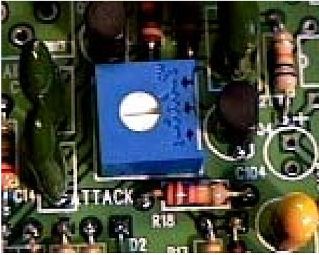
Inside the pedal, towards the top right on the circuit board is a TRIM POT labelled ATTACK.
