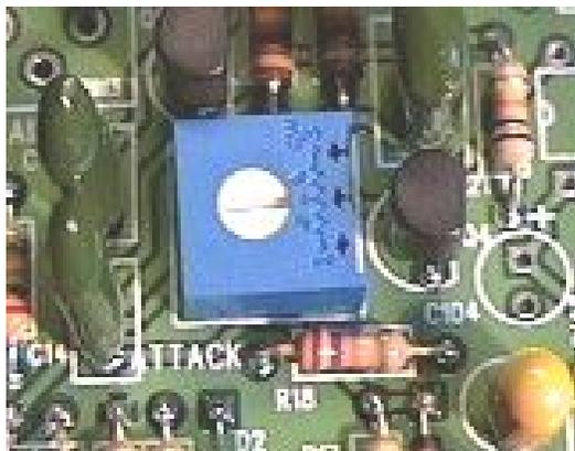
Inside the pedal, towards the top right on the circuit board is a TRIM POT labelled ATTACK. If the optional ATTACK KNOB is ordered, this applies to the external ATTACK knob instead.
